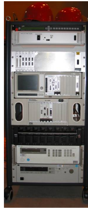
Figure 5-16: Control PC rack. From top to bottom: GPS receiver; LED pulser module; DSP interface module; Control PC; PCI extender; RAID array; FEE heaters power supply; FEE fans power supplies.
