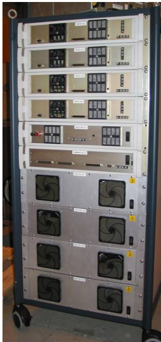
Figure 5-15: Digital Signal Processing rack. From top to bottom: four DSP modules; Magnet power supply; Temperature monitor and optical unit controller; Four low noise FEE power supplies.
